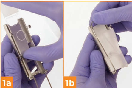
Place slide and funnel into metal clip and secure clip
