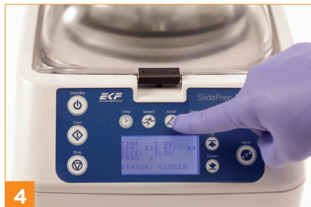
Install rotor head, close lid, select spin time, speed and acceleration then start spin
