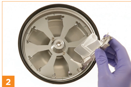
Load funnels into removable rotor head ensuring they are evenly balanced
