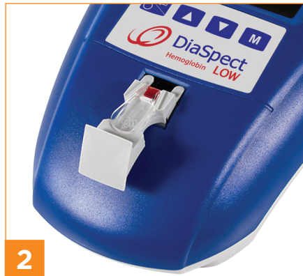
2 Insert cuvette and touch holder gently.
