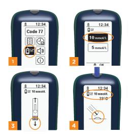
Move the measuring device with the inserted Test Strip to the droplet. Allow the droplet to fill the measurement chamber until the opening for the blood sample is immersed in the droplet. An acoustic signal will sound when the chamber has filled and the test will begin.
