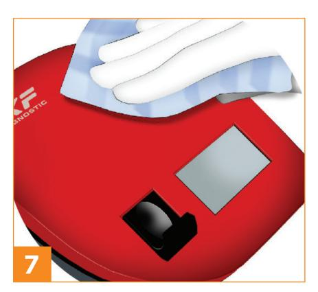
Cleaning of the housing and display is best accomplished with a lint-free cloth, lightly dampened with clear water or a mild soap solution. Commercially available, solvent and alcohol free solutions can be used for disinfection.
