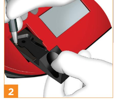
Open the cuvette holder until you feel a noticeable resistance. Press down the latch on the left-hand side of the cuvette holder with a pointed object and concurrently retract the cuvette holder to the front side.
