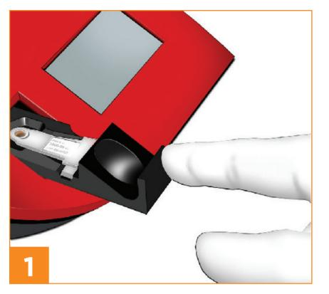
The optical unit should be cleaned at least monthly and if the control cuvette shows a deviating value, if control solutions cannot be measured correctly or if the error message "Dirty optics" is displayed.
