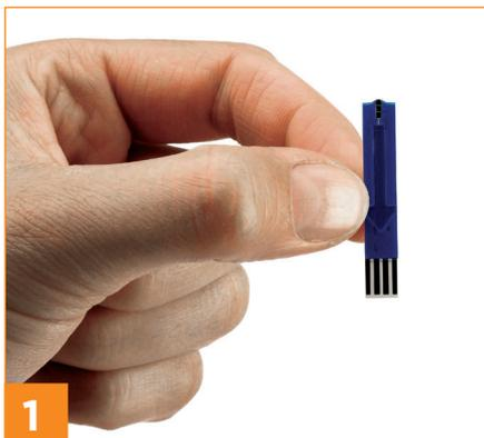
1 Remove sensor and place into analyser.
