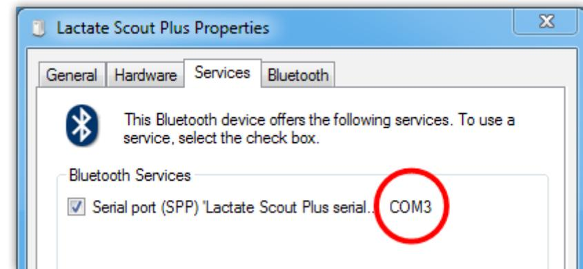
The COM port number shown in this window has to be entered at the communication settings of your software. Please read the appropriate section in the manual of the software you are using.
