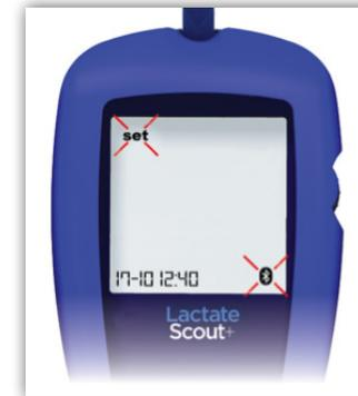
After pressing the scroll wheel briefly, the menu is activated and the message "OFF" is being displayed on the main display together with the blinking Bluetooth ®- icon:
