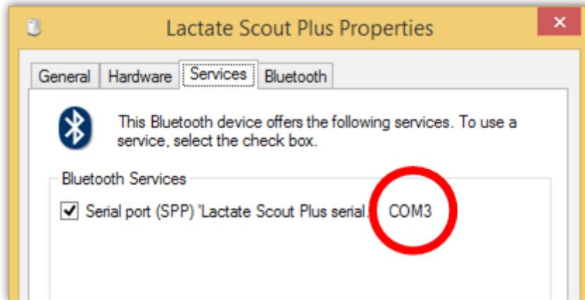
Now, the COM port number shown in this window has to be entered at the communication settings of your software. Please read the appropriate section in the manual of the software you are using.
