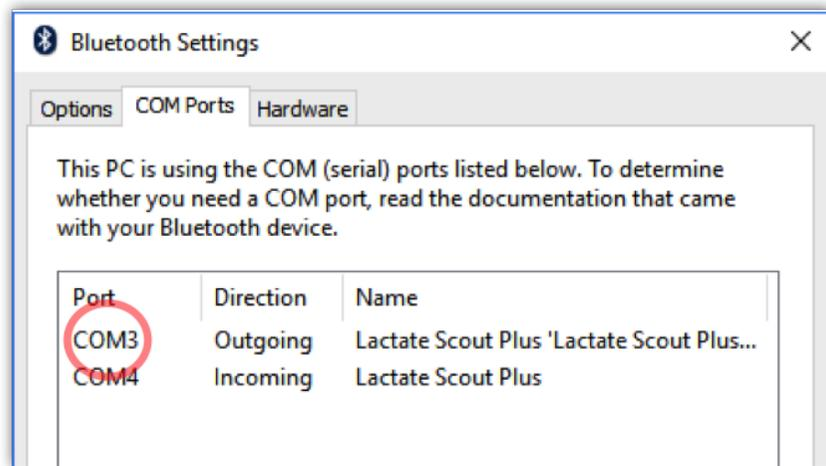
Now, the COM port number (Outgoing) shown in this window has to be entered at the communication settings of your software. Please read the appropriate section in the manual of the software you are using.
