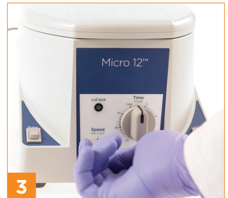
3 Close outer lid and select spin speed and spin time
