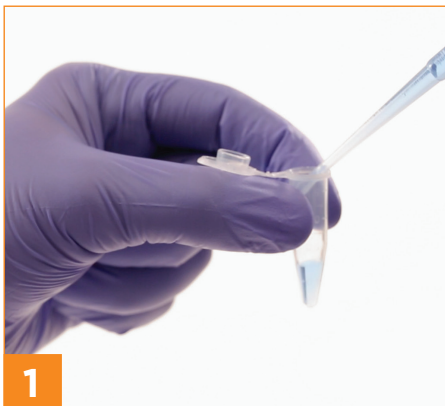
1 Pipette sample into tube and close cap tightly
