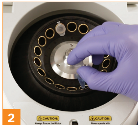
2 Place tube plus counterbalance tube (hinge facing up) into rotor and install inner lid.
