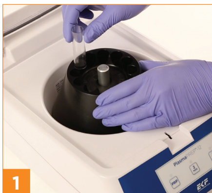
Insert tube holders into rotor.
