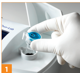
1 Scan lot calibration barcode. Remove foil from cartridge and insert into analyzer.
