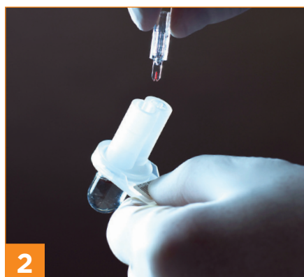
2 Insert sample collector into the Quo-Test cartridge.
