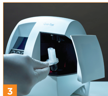
3 Insert cartridge into analyser. Results displayed within 4 minutes.
