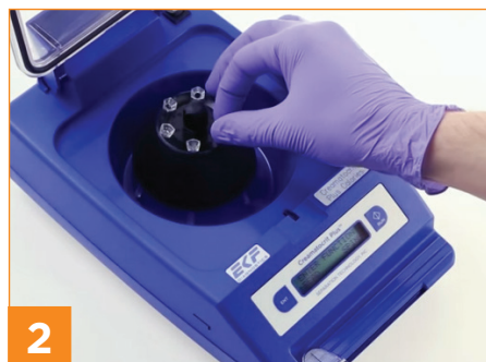
2 Seal the sample tube and place it into the centrifuge, ensuring rotor is evenly balanced. Shut lid and press RUN button.
