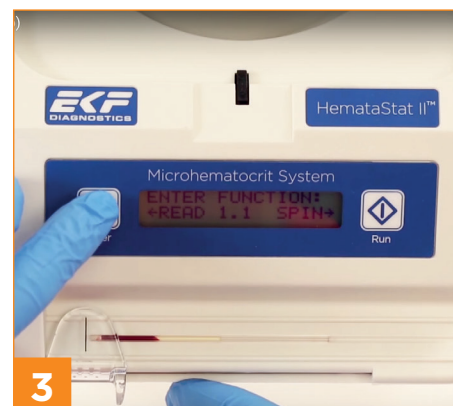
3 Read tubes on built-in reader tray. Results are displayed on screen.
