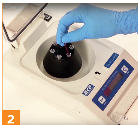
2 Seal the sample tube and place it into the centrifuge, ensuring rotor is evenly balanced. Shut lid and press spin button.
