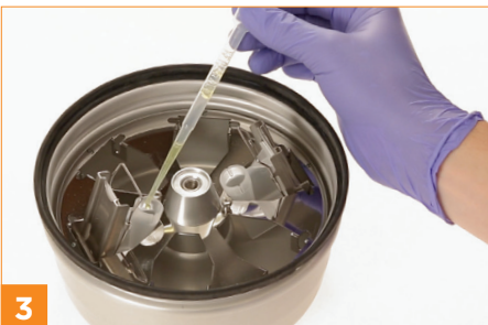
Pipette sample into funnel, install cap and secure bowl lid by tightening the knob
