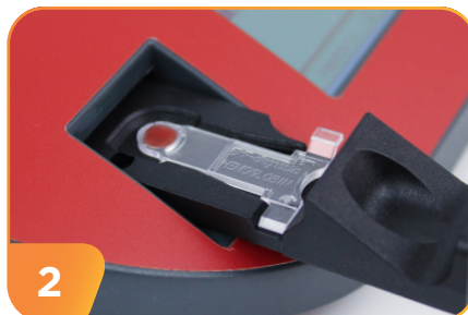
2 Put microcuvette into analyzer.
