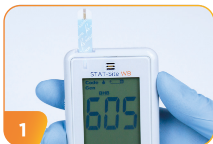
1 Insert test strip into the meter.
