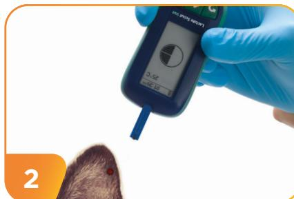
2 Position the tip of the Lactate Scout Test Strip on the sample site and collect blood by touching with test strip.
